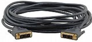
Kramer's C-MDM/MDM flexible DVI cables are high-performance cables with molded DVI-D connectors at both ends. These single link cables, designed to carry digital-only signals (18+1 pin), support signals up to 1920x1200 @60Hz and 1080p with 12-bit deep color. These cables are ideal for any installation or rack building that requires flexible cables
